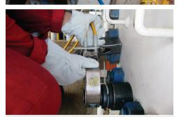
Quick couplings used on bolt tensioning equipment, hydraulic wrenches.
